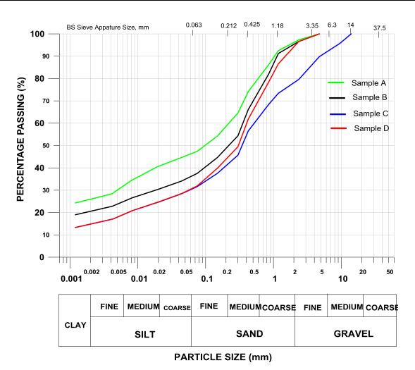
Figure 1 Grain size distribution curves for the soils
